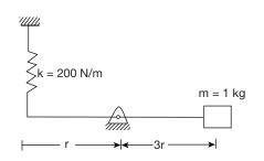
A thin uniform rod of mass 1 kg and length 4*r* is hinged at a distance r from one end as shown in figure and held horizontally. *A* point mass of 1 kg is at right end and a light spring of stiffness k = 200 N/m is at left end of rod. When the rod is slightly disturbed from its equilibrium portion, it undergoes vertical angular oscillations with a frequency (in rad/s) equal to
