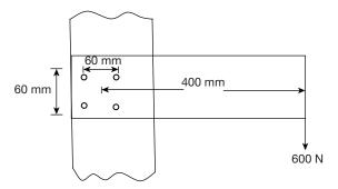
A horizontal plate has been joined to a vertical post using four rivets arranged as shown in figure. The
