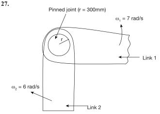
Figure shows a smooth pinned joint of pin radius r = 300 mm, connecting links 1 and 2 having angular velocities  $\omega_1 = 7$  rad/s counter clockwise and  $\omega_2 = 6$  rad/s clockwise as shown in figure. The velocity of rubbing at the pin joint (in m/s) is
