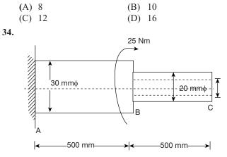
A stepped shaft ABC, fixed at A and hollow at portion BC is subjected to a twisting moment of 25 Nm at B. Shaft dimensions are as shown in the figure. Shear modulus G = 75 GPa. The angle of twist at C (in degrees) is .
