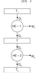
Two reversible heat engines HE-1 and HE-2 are connected in series and connected to thermal reservoirs at temperature  $T_1 = 1000$  K and  $T_3 = 300$  K as shown in figure. If the thermal efficiencies of the engines are
