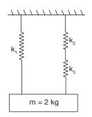
A mass of 2 kg is suspended by means of three springs as shown in figure. The spring constants  $k_1$ ,  $k_2$  and  $k_3$  are respectively 1 kN/m, 2 kN/m and 3 kN/m. The natural frequency of vibration of system is approximately (in rad/second)
