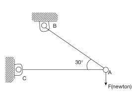
In the arrangement shown links AB and AC are uniform, made of same material, having same lengths and same areas of cross-section. When joint A is pulled down by a force F newton,  $|\Delta L_1|$  and  $|\Delta L_2|$  are the
