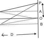
at O in the same phase. So O is bright fringe. Let waves coming from  $S_1$  and  $S_2$  meets at screen at point P at a distance y from central fringe.
