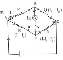
Let P, Q, R, and S be four resistors, Let P, Q, R are known and S is unknown. Adjust P, Q, R so that galvanometer shows no deflection by closing key K.
