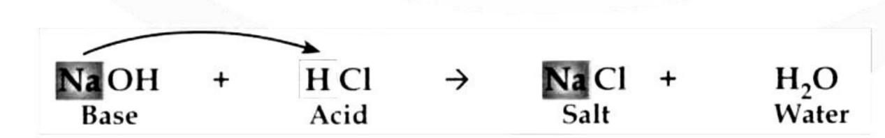
REPLACEMENT OF H<sup>+</sup> ION OF THE ACID The hydrogen ion 1H<sup>+</sup>J aq. of the acid is replaced by the metal atom (Na<sup>+</sup>) of the base - forming a salt - NaCl.
