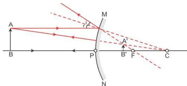
A concave mirror can form a magnified and virtual image. A convex mirror cannot form an enlarged image. When the object is placed between the pole and the focus of the mirror, the image formed is virtual, enlarged and erect.
