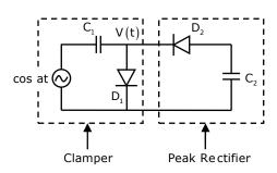
When excited by cos ( $\omega t$ ), the clamping section clamp the positive peak to 0 volts and negative peak to -2 volts. So whole  $\cos(\omega t)$  is lower by -1 volts
