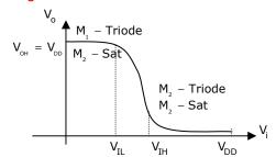
where  $V_{IL}=\frac{1}{8}(3V_{DD}+2V_{t})=2.125V$  , Hence Option 'A' is approximately correct.
