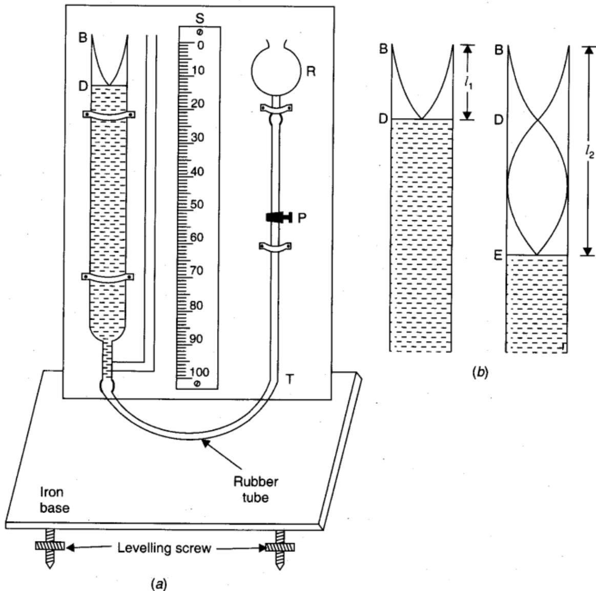
**Fig.** Resonance tube.
