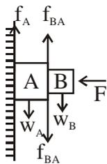
F is provide the normal force. Weight of A & B in downward direction. So friction force  $f_A$  &  $f_{BA}$  (friction B due to A) is upwards direction.
