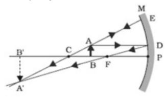
iv. Yes, concave mirror can be used to obtain a diminished image. When the object is placed beyond 2f, then the image formed will be diminished one.
