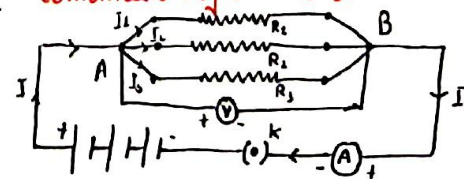
$$\text{Total Current flowing } I = I_1 + I_2 + I_3$$
