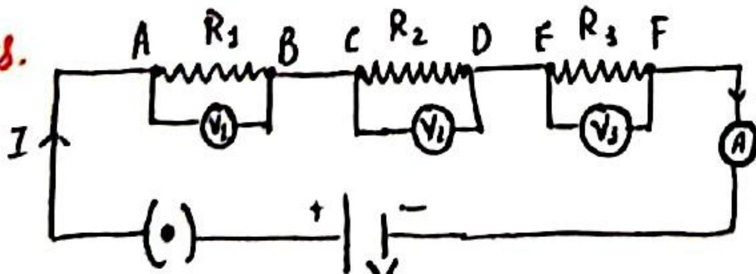
$$\text{Total potential difference } (V) = V_1 + V_2 + V_3$$
