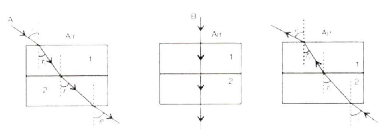
Speed of light in medium '1' is less than speed of light in medium '2'.
