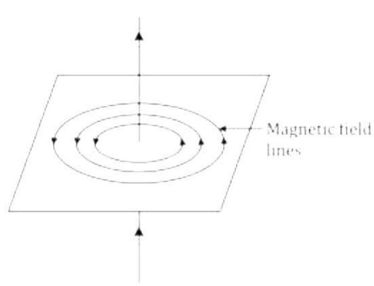
(b) The Right-hand thumb rule was used to find the direction of magnetic field lines.
