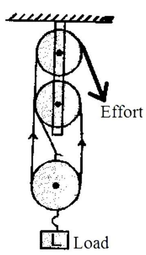
If w be the total weight of the pulleys in the lower block, in the balanced position
