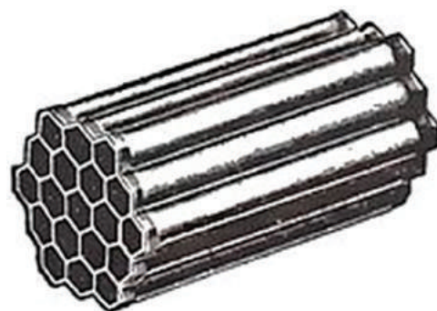
Fig 7.3.1(b) Honey comb type radiator
