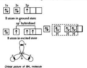
B atom gets hybridized to form three equivalent hybrid orbitals directed towards three corners of an equivalent triangle with B atoms in the center. Bond angle = 120°.
