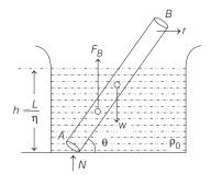
If the rod is in equilibrium, then the net torque about the point  ${\cal A}$  is zero i.e.
