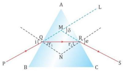
As the ray PQ after refraction from surface AB emerges from face AC at point R of the prism, it implies that the refracted ray QR travels parallel to the base of the prism. This happens at the minimum deviation position.
