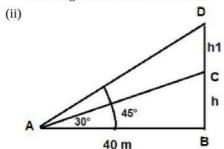
Let BC be the tower of height h and CD be the water tank of height  $h_1$
