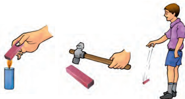
Fig. 13.15 Magnets lose their property on heating, hammering and dropping
