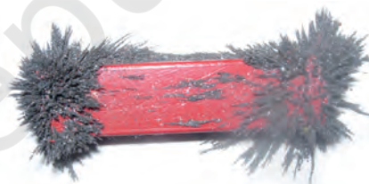
Fig. 13.7 Iron filings sticking to a bar magnet
