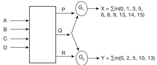
Assuming that  $G_1$  is NAND gate, and  $G_2$  is AND gate, find the smallest function 'Q'. (with minimum number of min terms) which makes it possible to produce  $X$  and  $Y$ ?
