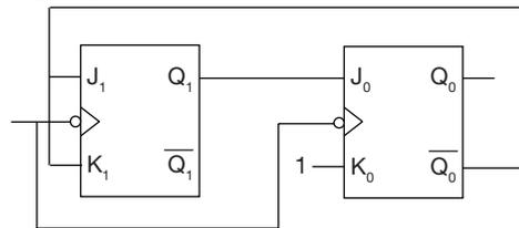
If the JK flip flops have to be replaced by  $D$  flip flops, for the same sequence then the  $D$  flip flop inputs  $D_1, D_0$  are (corresponding to  $Q_1, Q_0$  flip flops)
