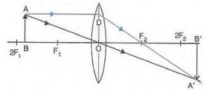
The image formed in above diagram is real, enlarged and inverted.
