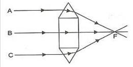
As shown in the figure the convex lens has two glass prisms and one glass block. One of the glass prisms is situated above the glass block and one below the block.
