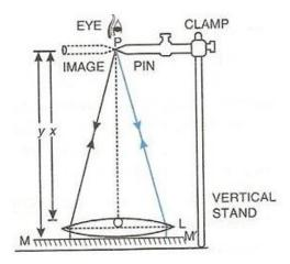
Adjust the height of the pin until it has no parallax (i.e., when the pin and its image shift together) with its inverted image as seen from vertically above the pin.
