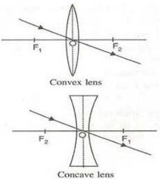
(ii) A ray of light incident parallel to the principal axis of the lens, after refraction passes through the second focus F<sub>2</sub> (in a convex lens) or appears to come from the second focus F<sub>2</sub> (in a concave lens).
