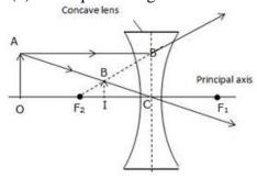
(c)The focal length is measured from optical centre C to F<sub>2</sub>.
