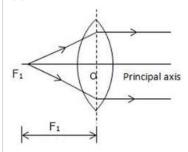
(b) The point where incident ray passes through a point on the principal axis is called first focus.
