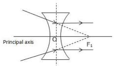
The second focal point for a concave lens is a point  $F_2$  on the principal axis of the lens such that the rays of light incident parallel to the principal axis, after refraction from the lens, appear to be diverging from this point.
