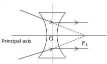
(b) The point where incident ray when produced meets the principal axis is called first focus.
