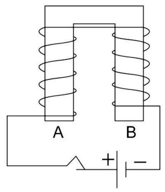
Diagram showing a coil wound around a U-shape soft iron bar AB.
