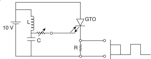
A 10 volt pulse generator made by using GTO  $L = 0.1$  H.,  $C = 10 \mu$ F.
