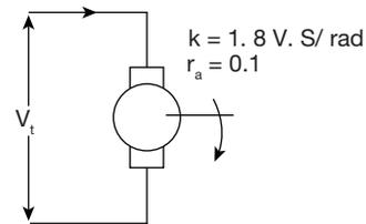
At no load armature current of 25 A what will be the no load speed at firing angle of  $45^\circ$ .
