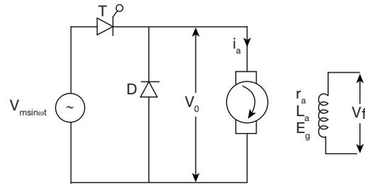
A single phase DC motor drive as shown which of the following is right for the circuit on the assumption of  $La \gg ra$ .
