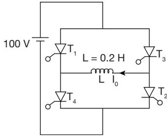
Operated in  $180^\circ$  mode, 50 Hz the peak to peak value of  $I_o$  will be
