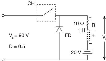
The circuit having chopping frequency of 1500 Hz. What will be the maximum ripple current flow through the inductor
