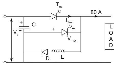
Commutation circuit as shown in figure having  $L = C = 1 \text{ m}$  units and  $V_c = 120 \text{ V}$  maximum voltage a capacitor can store. What will be the minimum current main thyristor can be handling.
