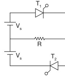
Inverter arrangement as shown in figure having  $V_s = 100 \text{ V}$  and  $R = 10 \text{ W}$  what will be the maximum value of 5<sup>th</sup> harmonic component.
