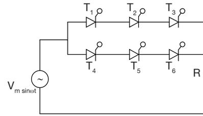
6 identical switches of forward voltage handling capability of  $V_{\max} = 400$  rms
