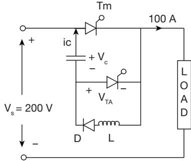
Having  $L = 20 \mu\text{H}$  and  $C = 50 \mu\text{F}$ ,  $V_c = V_s$  for a constant load current of 100 A. What will be turn off time for main thyristor  $T_m$
