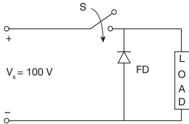
The circuit as shown with duty cycle of switch,  $D = 0.5$  will follow
