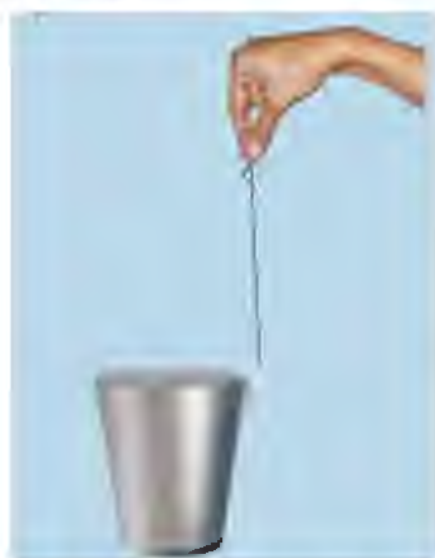
Fig. 5.17 : Thermocole Ball Touching the Vibrating Glass Tumbler
