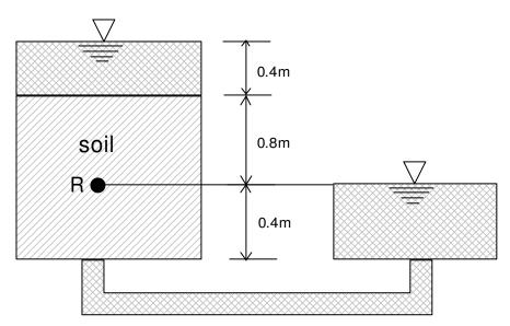
Q.70 The total head, elevation head and pressure head in metres of water at the point R shown in the figure are
