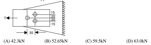
Q.42 A bracket connection is made with four bolts of 10mm diameter and supports a load of 10kN a an eccentricity of 100mm. the maximum force to be resisted by any bolt will be
