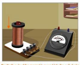
The North pole of the magnet is moved into the coll of wire
