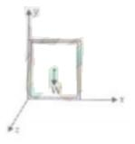
Here axis of rotation of door is along Y-axis and door is in x-y plane and force F can be applied along  $\pm$  z-axis, the torque is experience by door. So a force can produce torque
