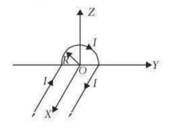
Linear parts of the wire are very long and parallel to X-axis while semicircular portion of
