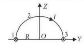
Parallel wires 1 and 3 are semi-infinite, so magnetic field at *O* due to them
