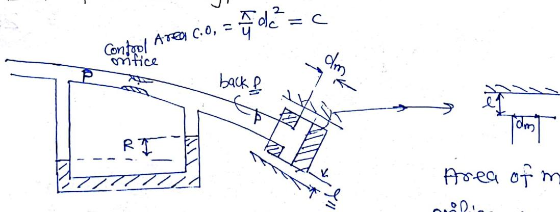
Area of measuring orifice  $M = \pi d_m l$
