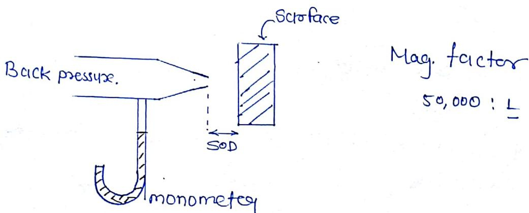
Pneumatics Comparators work on the principle of an air jet i.e. when we try to block the orifice, due to loss of momentum pressure will develop on the back ground of jet.
