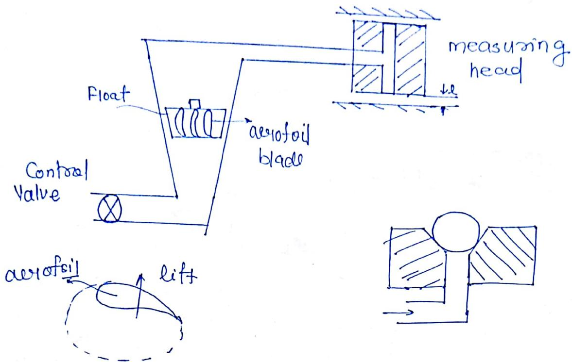
Measuring heads are designed according to the geometry of work.
