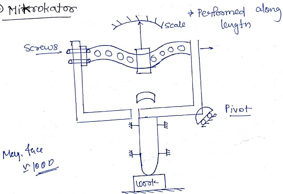
A thin sheet is given Right hand twist on Right side and left hand twist on left side centre is Neutral. If the sheet is too thin there will be plastic deformation during twist and if the sheet is too thick there will be development of residual stress.
