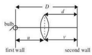
Now, we know that to form a real image of an object on a screen by a convex lens, the distance between the source and the screen (D) should be equal to 4f, where f is the focal length of the lens.
