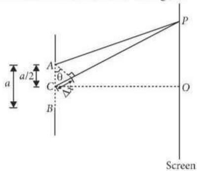
In figure A and B represent the edges of the slit AB of width a and C represents the midpoint of the slit. For the first minimum at P,
