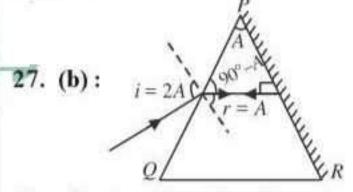
On reflection from the silvered surface, the incident ray will retrace its path, if it falls normally on the surface.
