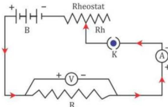
A – Ammeter (used to measure electric current)
