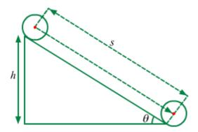
The body is at rest at the top of the inclined plane. Now, let the moment of inertia of the body be I, v be the linear speed and  $\omega$  be the angular speed acquired by the body when it reaches the bottom of the inclined plane.
