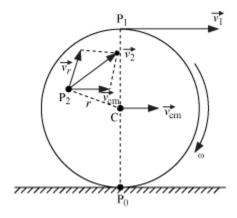
At any instant, the point of contact  $P_0$  of the disc with the surface is at rest.
