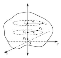
In rotation of a rigid body about a fixed axis, every particle of the body moves in a circle, which lies in a plane perpendicular to the axis and has its centre on the axis.
