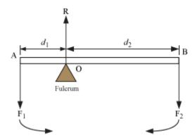
Here,  $F_1$  and  $F_2$  are two parallel forces. R is the reaction of the support at the fulcrum.
