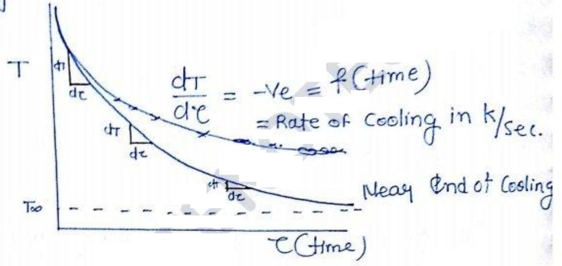
\* During unsteady state H.T. the rate of cooling or heating of body it self becomes a function of time initially the rate of cooling is very high due to high convection H.T. Rate between body and fluid because of large temp. diff. b/w them. but as the time progresses this rate of cooling decreases due to reducing H.T. rate b/w body and fluid because of lesser temp. diff. between them.
