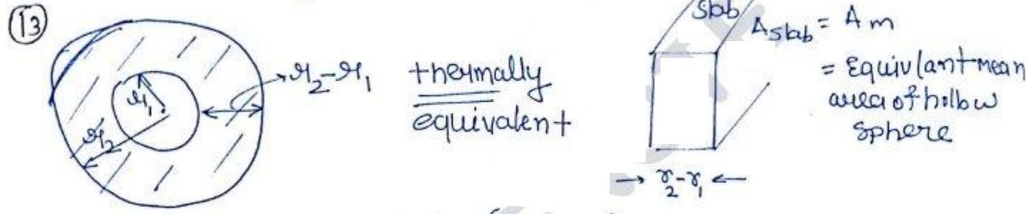
$$R_{th} = \frac{r_2 - r_1}{4\pi k r_1 r_2}$$
