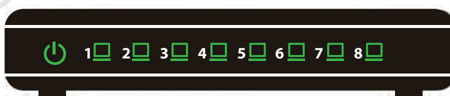
Figure 5.8: A network hub with 8 ports
