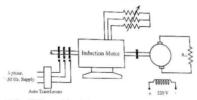
The motor is coupled to a 220 V, separately excited. dc generator feeding power to fixed resistance of  $10~\Omega$ . Two-wattmeter method is used to measure the input power to induction motor. The variable resistance is adjusted such that the motor runs at 1410 rpm and the following readings were recorded
