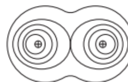
Equipotential surfaces due to two positive charges
