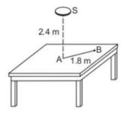
**Solution:** Given: Illuminance at A = 25 lux. Form figure, AS = 2.4 m and AB = 1.8 m.
