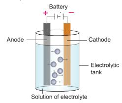
Figure 16.2 Electrolytic Cell
