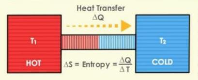
This law states that energy naturally flows from hotter objects to cooler objects. In order for energy to flow from a cooler object to a hotter object, work must be done. When heat is converted into work, the efficiency or output of usable work will always be less than 100%.
