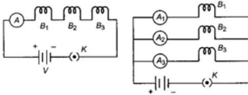
Equivalent resistance in series combination  $R_s = R + R + R = 3R$ , Voltage = V
