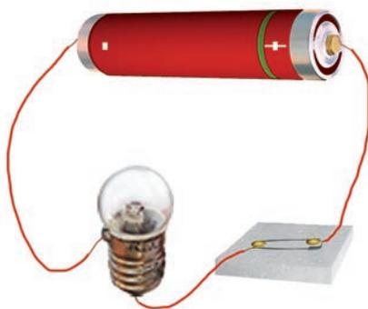
11. No the bulb will not glow in this circuit because the switch is open and the circuit is incomplete.
