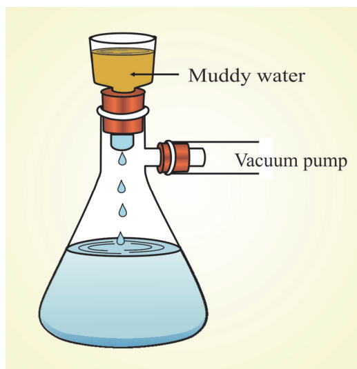
Fig. 2.13: Filtration (a) simple filtration (b) vacuum filtration
