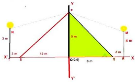
In the left and right side of the pole, two street lights are fixed at a height of 3m and 4m respectively. These lights are given supply by wires PM and PN. The height OP=5 m and O is the origin.
