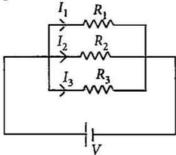
The current flowing through the two resistances in parallel is, however, not the same. When we have two or more resistances joined in parallel to one another, then the same current gets additional paths to flow and the overall resistance decreases.
