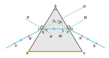
PE – Incident ray $\angle 1$  – Angle of incidenceEF – Refracted ray $\angle r$  – Angle of refractionFS – Emergent ray $\angle e$  – Angle of emergence $\angle A$  – Angle of the prism $\angle D$  – Angle of deviation
