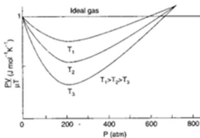
Experimentally value of  $\frac{PV}{\mu T}$  for real gas was calculated by altering the pressure of gas at different temperatures. The graphs obtained have been shown in the diagram. Here for the purpose of comparison, graph for an ideal gas has also been drawn, which is a straight line parallel to pressure axis.
