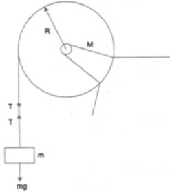
Where a is the tangential acceleration of appoint on the rim of the disc.
