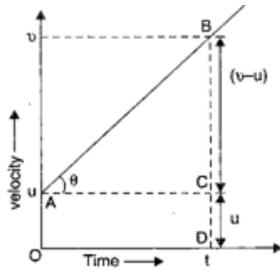
Let  $u$  be the initial velocity of the particle at  $t = 0$  and  $v$  is the final velocity of the particle after time  $t$ . Consider two points  $A$  and  $B$  on the curve corresponding to  $t = 0$  and  $t = t$ .
