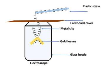
**Tip:** Remember when a person touches the top of the metal clip, the foil strips converge or they come back to their original state. This has happened because the charge on the foil strips loses charge to the earth through the person's body and there is no repulsion between the foil strips.
