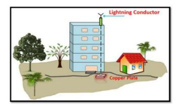
**Tip:** The lightning conductor is always taller than the building.
