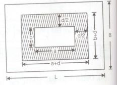
Net punching force Punching shear stress developed = cross-section area of resisting section
