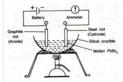
**Reaction at cathode**: Lead ions are positively charged they get discharged at cathode. It receives two electrons from cathode and changes to atom of lead and get deposited at the cathode.
