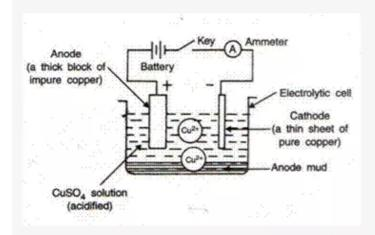
Therefore there is transference of copper atoms from anode to cathode.
