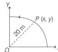
The movement of  $p$  is such that it sweeps out a length  $s = t^3 + 5$ , where,  $s$  is in metre and  $t$  is in second. The radius of the path is 20 m. The acceleration of  $P$  when  $t = 2s$  is nearly
