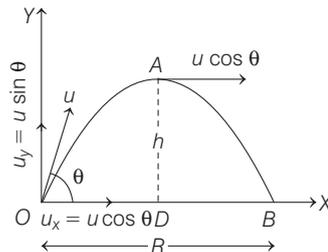
Let a particle is projected at an angle  $\theta$  from the ground with initial velocity  $u$ .
