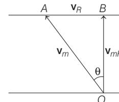
In  $\Delta OAB$ ,  $\sin \theta = \frac{v_R}{v_m}$  and  $v_{mR} = \sqrt{v_m^2 - v_R^2}$
