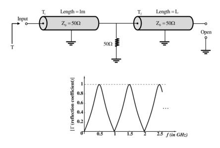
The length L (in meters) of T<sub>2</sub> is \_\_\_\_\_
