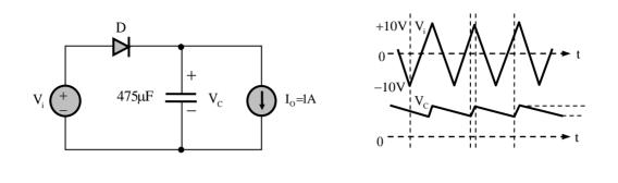
The value of the ripple V (in volts) is \_\_\_\_\_.
