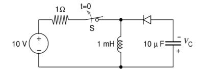
The steady state magnitude of the capacitor voltage  $V_C$  (in volts) is \_\_\_\_\_. Answer: (100)
