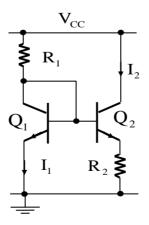
The bipolar transistors  $Q_1$  and  $Q_2$  are perfectly matched and have very high current gain, so their base currents are negligible. The supply voltage  $V_{cc}$  is 6 V. The thermal voltage kT/q is 26 mV.
