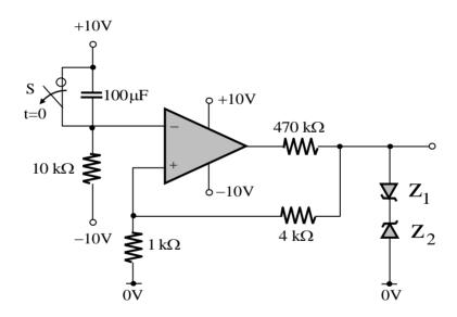
The time  $t = t_1$  (in seconds) at which  $V_0$  changes state is\_\_\_\_\_.
