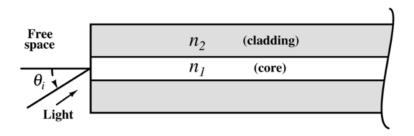
The maximum value of  $\theta_i$  (in degrees) for which the incident light will be guided in the core of the fibre is \_\_\_\_\_.
