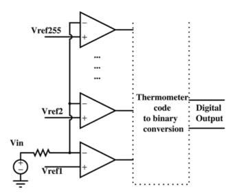
The input must settle to an accuracy of 1/2LSB even for a full scale input change for proper conversion. Assume that the time taken by the thermometer to binary encoder is negligible.
