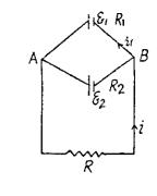
Thus one can replace the given arrangement of the cells by a single cell having the emf  $\xi_0$  and internal resistance  $R_0$ .
