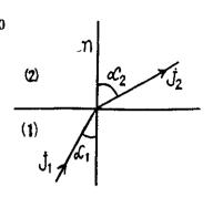
3.165 The electric field in conductor 1 is
