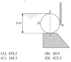
**22.** The maximum downward acceleration of the vessel if cavitation should be avoided will be  $(P_{\text{saturation}} = \text{Vapour pressure} = 2.8 \text{ m of water (absolute) and atmospheric pressure} = 100 \text{ kPa})$
