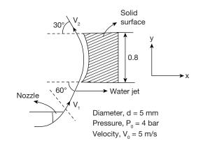
The force exerted on the solid body in x direction by the jet in (N) will be
